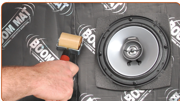
Adding Boom Mat damping material to the speaker mounting surface reduces vibrations and improves acoustics.
