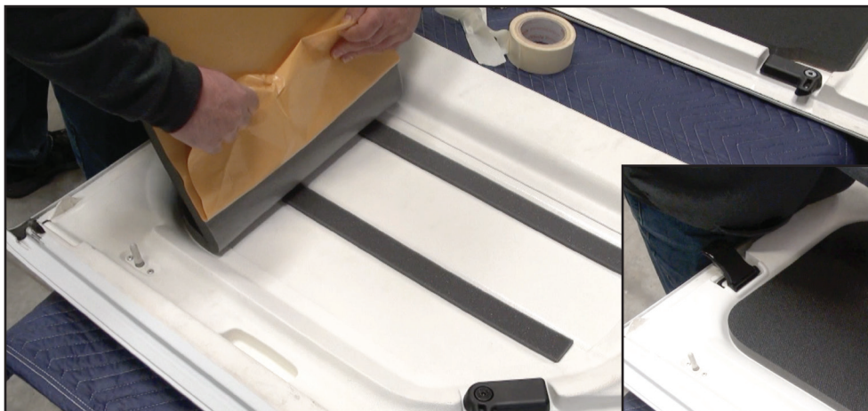
FIG. 7 & Fig 8 Slowly pull the release liner off as you press the piece into place. NOTE: Use gentle pressure. DO NOT use a lot of pressure when pressing piece into place.
