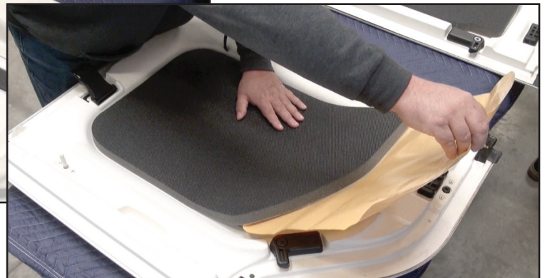
FIG. 7 & Fig 8 Slowly pull the release liner off as you press the piece into place. NOTE: Use gentle pressure. DO NOT use a lot of pressure when pressing piece into place.
