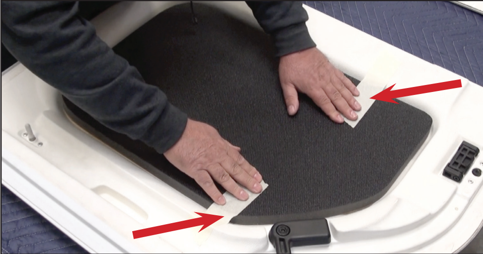
FIG. 5 Align piece in freedom top and use a mild tape to temporarily hold in place.
