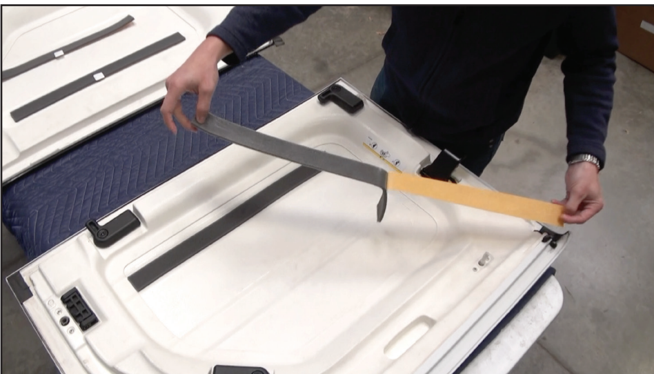
FIG. 4 Peel the backing off filler strips and place into grooves.
