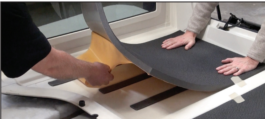
FIG. 10 Peel back a small section of release liner start to adhere the piece to the top. Continue to pull the release liner off and gently press piece in place
