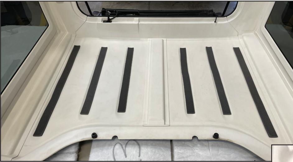
3.) Test fit the filler strips into the ribs of corresponding length before peeling the release liner on the strips. Refer to proper diagram on page 2 for proper placement of filler strips.
