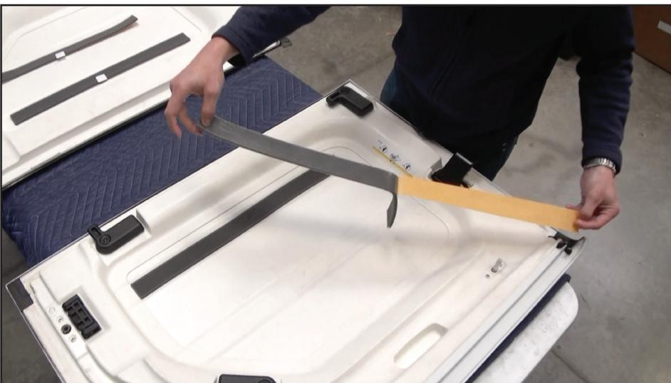
4.) Install the foam “filler strips” in the molded ribs to ensure a smooth installation of the headliner. Without the “filler strips”, the headliner will conform to the ridges in the top leaving an uneven appearance.
