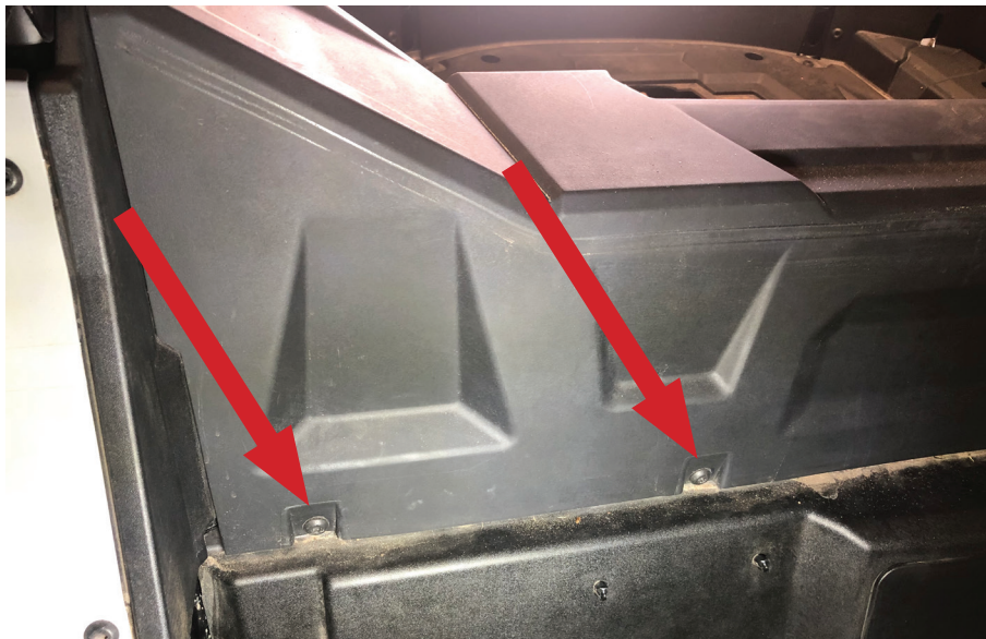
Fig. 5 - This image shows 2 screws on passenger side that need to be removed. There are also one on the driver side that need removed as well.
