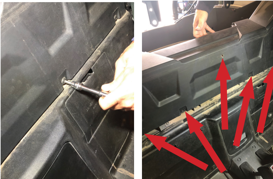
Fig. 3 - Remove 5 torx screws holding upper panel behind seats
