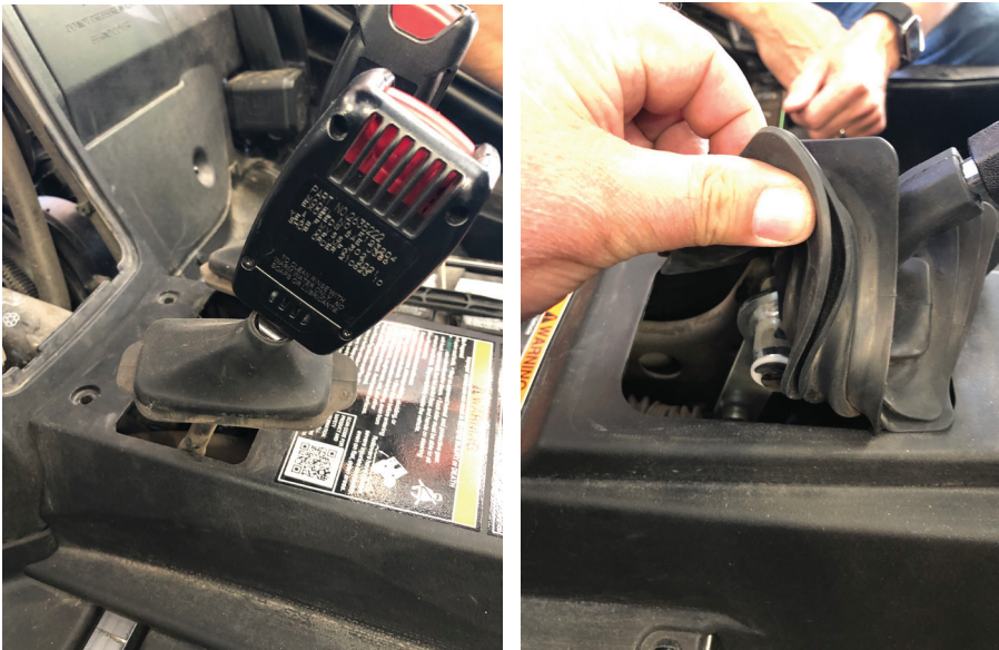
Fig. 8 - Push rubber boots through openings as you lift out center console
