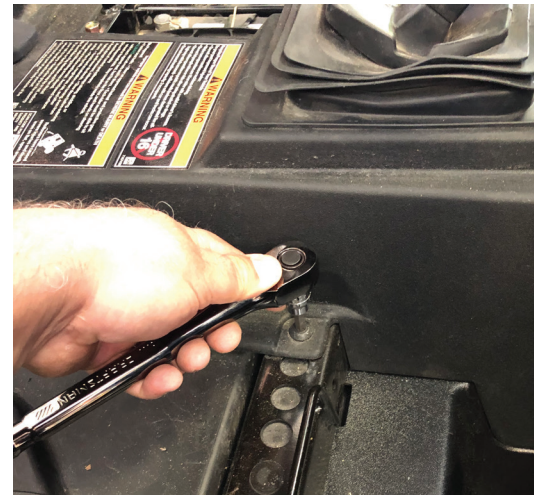
Fig. 6 - Driver side screw to be removed
