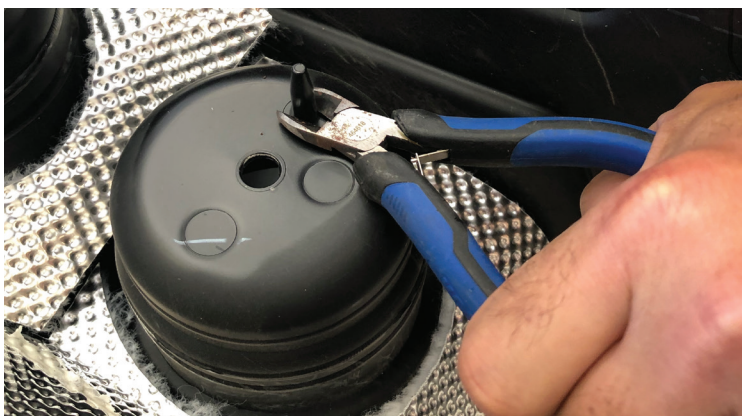
Fig. 10 - Clip off tabs on the bottom side of both cup holders
