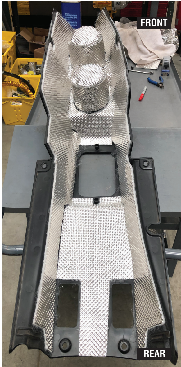
Completed installation of console insulation
