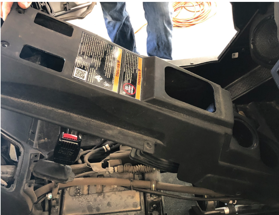
Fig. 9 - Lift out center console
