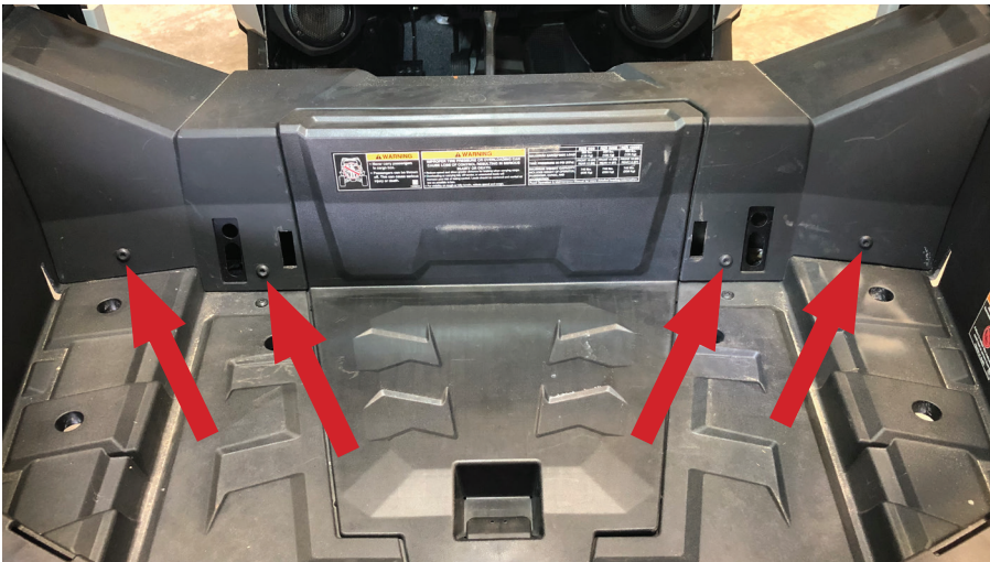
Fig. 2 - Remove 4 torx screws holding front bed cover
