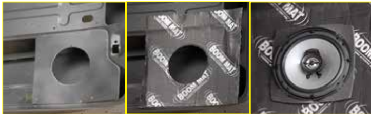
Remove speaker, apply material, re-install speaker
