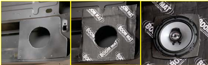
Remove speaker, apply material, re-install speaker
